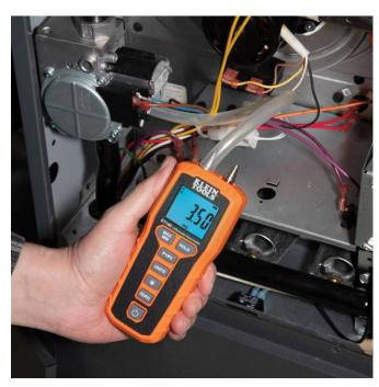
as identifying pressure drops at filters and pressure loss in ducts. Tapered ports allow for a variety of tubing size attachments, and the magnet on the back allows professionals to free up their hands for easier operation."
