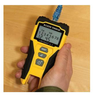
"Klein Tools' new LAN Scout Jr. 2 Data Cable Tester is the next generation of cable testing, designed to take all the functionality from the last LAN Scout Jr. Tester and improve upon it," says Karen Alpan, product manager at Klein Tools. "With the larger backlit LCD screen, more intuitive three button interface as well as the switch from button batteries to AAAs, this tester makes testing data cables guicker and easier for professionals."
