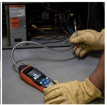
"Klein Tools engineered the ET160 to easily detect refrigerant gases with both audible and visual alarms in the presence of CFCs, HFC, HCFCs and blends," says Sabrina Kalsi, product manager at Klein Tools. "The 18" gooseneck probe allows for easy access around equipment, and useful features like automatic zero-point calibration, hold, mute and low battery indicator mean that this detector is ideal for troubleshooting and maintenance of air conditioning and refrigeration units."
