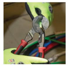
"Klein Tools' team engineered the new High-Leverage Cable Cutter to require 30% less force to cut aluminum, copper and communications cable as compared to previous Klein Tools' models," says Jeff Meek, director of product management at Klein Tools. "The integrated stripping hole strips 1/0 and 2/0 cable making it easier for trade professionals to get the job done with less tools."
