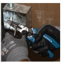
"Designing this tool, we wanted to bring together the durability of pliers, the sharpness and precision of a wire stripper and an integrated crimper," says Jeff Meek, director of product management and development at Klein Tools. "This stripper and crimper brings together six of the most commonly used stripping holes along with a crimper, giving users the convenience of using one tool for multiple tasks, saving them the time and effort of switching tools in the middle of a job."
