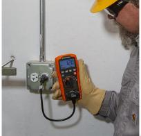
combines multiple core electrical products into one convenient tool. It is an auto-ranging digital multi-tester that measures AC/DC voltage, resistance, continuity, and performs a battery test. It also tests wiring conditions in standard 120VAC and GFCI electrical receptacles and inspects North American GFCI devices."
