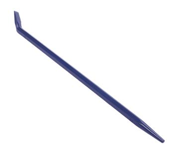
Used for levering and aligning, this podger bar is forged from tough high-tensile carbon manganese steel for maximum performance. The heel is set to 40-degree angle for optimum levering while the blade is ground to 30-degree angle for easy entry between surfaces. The taper is forged, not turned, for finer grain, giving greater tensile strength. The hexagonal profile provides greater control and minimizes bar roll.
