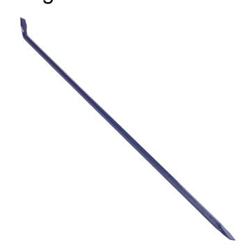
Used to lever and move objects into place with a lift and swivel motion. The hexagonal bar profile gives greater control and reduces bar roll. Forged from high-tensile carbon manganese steel for maximum strength. The heel is offset to 40° angle for optimum lifting.
