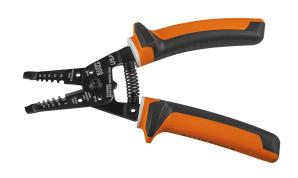
Klein Tools Electrician's Insulated Solid and Stranded Stripper is 1000V rated and VDE certified for safety on the job. The multi-color, sleek design with small thumbguards make for easy handling and storage. The three-part insulation with white underlayer provides a warning sign that insulation may be compromised. The durable, molded insulation meets or exceeds IEC 60900 and ASTM F1505 standards for insulated tools.
