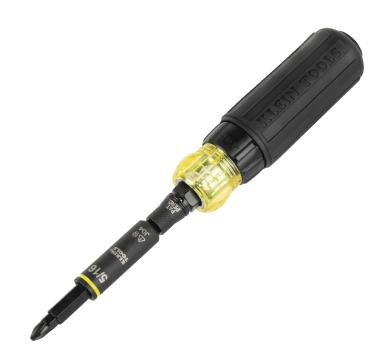
The Klein Tools 11-in-1 Ratcheting Impact Rated Screwdriver / Nut Driver's components are all impact rated for use with an impact driver. 1/4-Inch quick-connect on power nut drivers to easily switch from screwdriver handle to an impact driver (Impact driver not included). Ratcheting feature has three settings: forward, fixed, and reverse, facilitating easier driving.
